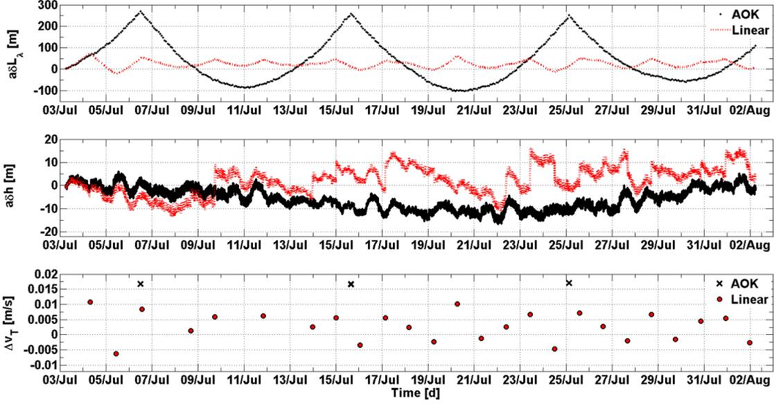
**Figure 3.** Phase and altitude differences at the AN and executed orbital maneuvers
