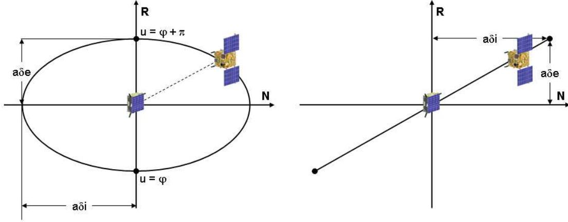
**Figure 1.** Projection of relative motion in the cross-track/radial plane for parallel (left) and orthogonal (right) relative  $e/i$ -vectors [6]
