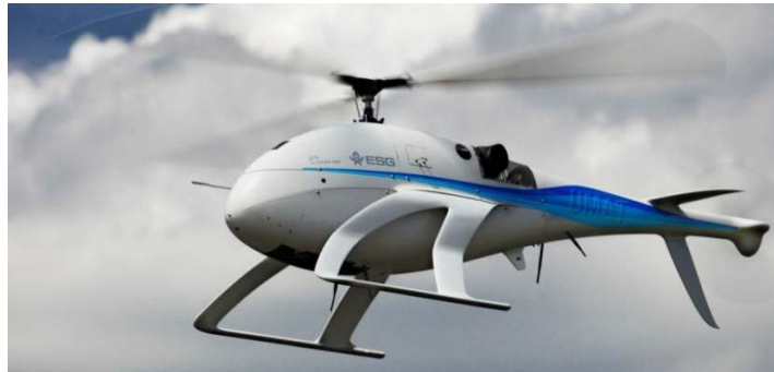
Figure 6. ESG's unmanned mission avionics test helicopter.
