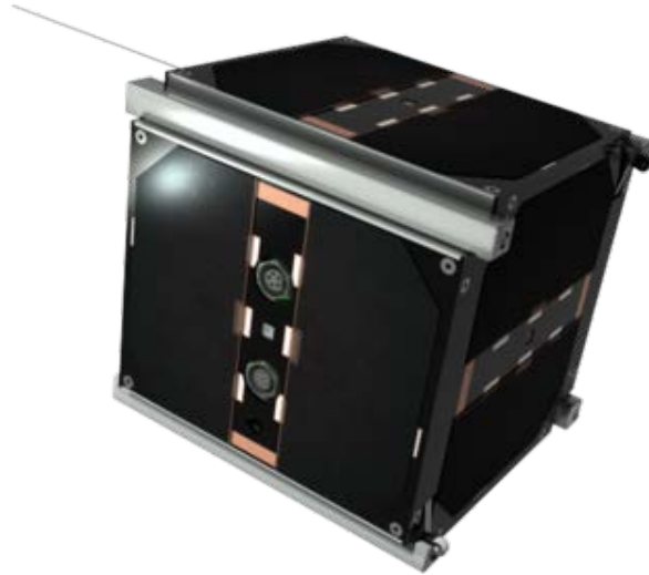
Figure 4. UWE-3: Picosatellite of the University of Würzburg
