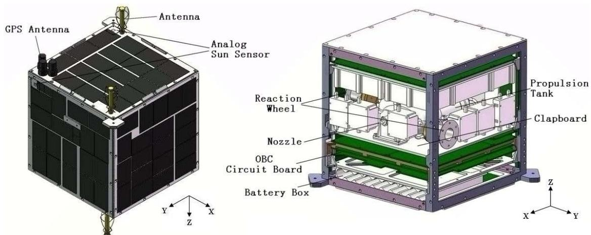
**Figure 2. View of the external (left) and internal (right) ZDPS-2 Structure**
