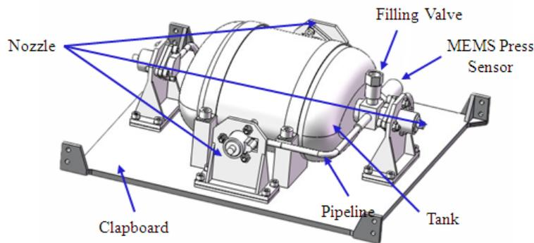
**Figure 3. ZDPS-2 Ammonia Propulsion System Structure**
