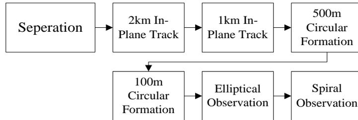
**Figure 4. Entire ZDPS-2 Formation Demonstration Procedure**
