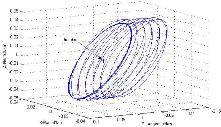
**Figure 7. Relative Motion of ZDPS-2 Spiral Observation**
