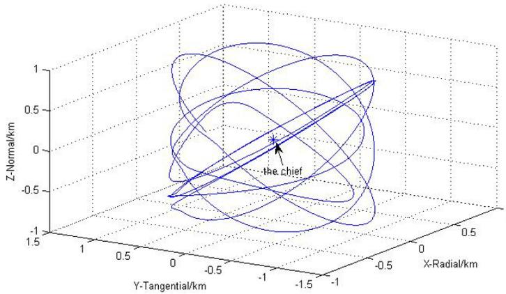
**Figure 6. Relative Motion of ZDPS-2 Elliptical Observation**
