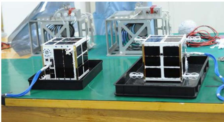
**Figure 1. View of the integrated ZDPS-1A Satellites with its disengaging gear**
